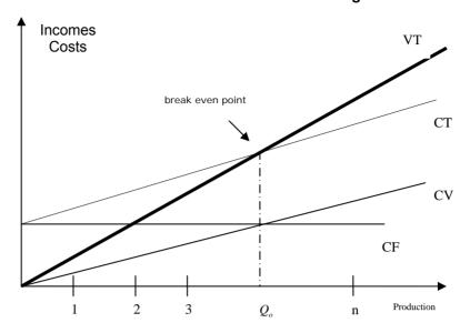
This way of determinating the break even point is made according to the volume of production, incase of linear evolution of the prices and variable costs.
